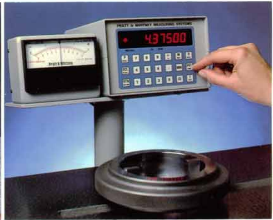
Zeroing the analog meter & printing the measurement
